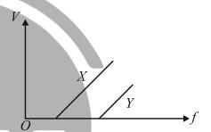
Greater work function means more negative potential is required to stop the ejection of electrons. Moreover, the slope of both the graphs will be the same.
