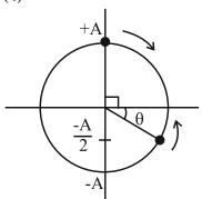
From the figure we can see that ' $\theta + 90^{\circ}$ ' is the phase angle here.
