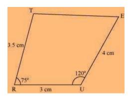
(1) Draw a line segment RU of 3 cm and an angle of 120° at point U. As vertex E is 4 cm away from vertex U, cut a line segment UE of 4 cm from this ray.
