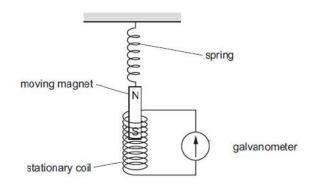
A magnet is attached to a spring. The magnet can go in and out of the stationary coil.
