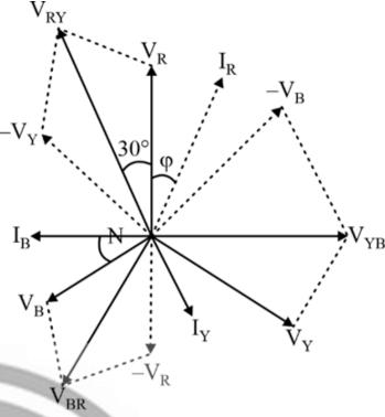
The angle between line voltage and phase voltage is  $30^\circ$  (angle between phase  $V_R$  and line voltage  $V_{RY}$ ) as shown above in the above diagram. In star connection line current is equal to phase current. Therefore, angle between line currents and the corresponding line voltages is  $30^\circ + \emptyset$  for lagging.
