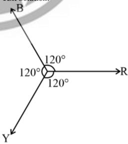
In balance system the three component are equal in magnitude and have 120° phase difference.
