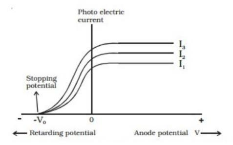
Electrons are released and visible light is absorbed by the photosensitive plate, also known as the emitter. All of the electrons that are released by the emitter are collected by the metal plate (collector). A photoelectric current flow results from this (from emitter to collector). This is consistently in opposition to the electrons' directions. A voltmeter and current probe can be used to measure the potential difference (V) and current (I) between the plates.
