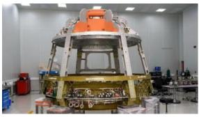
This system employs 12 thrusters, each with a 100N capacity, along with a pressurisation system with high pressure gas bottles and the propellant feed system along with the associated fluid control components.
