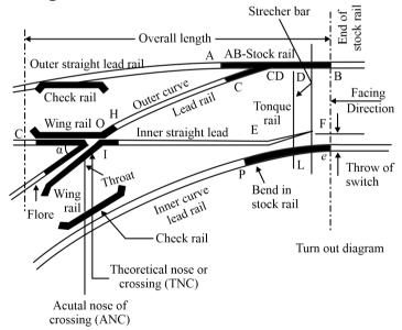
**Stock rail:** The running rail against which the tongue rail operates is called the Stock rail.
