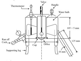
2. Softening point test Ring and ball apparatus are used to fine softening point. It is the temperature at which the bitumen attains a particular degree of softening. The diameter of steel ball is 0.95 cm, constant 5-6°C temperature is increased per minute. It is conducted at 35 to 70°C
