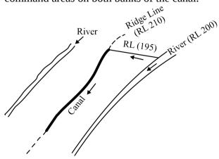
Contour canal aligned nearly parallel to the contours of the area, irrigation possible on one side of the canal only.
