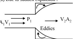
$$h_{L} = \frac{(V_1 - V_2)^2}{2g}$$
