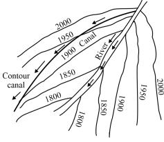
Side slope canal is constructed at right angles to the contours & does not intercept any cross drainage.
