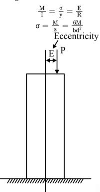
Eccentricity loaded column Then bending stress =  $\frac{6M}{bd^2} = \frac{6 \times P \times e}{bd^2}$   $\sigma = \frac{6 \cdot Pe}{bd^2}$
