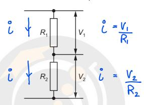
What is the relationship between  $R_1$ ,  $R_2$  and potential differences  $V_1$  and  $V_2$ ?
