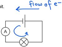
In which direction do free electrons flow around this circuit and what quantity does the ammeter measure?
