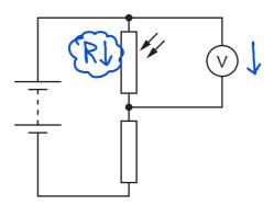
The brightness of the light falling on the LDR is increased.
