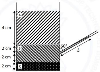
At the operating temperature and pressure, the specific gravities of liquids A, B and C are 1, 2 and 4, respectively. Neglect any surface tension effects in the calculations. The length of the tube L that is wetted by liquid B is cm.
