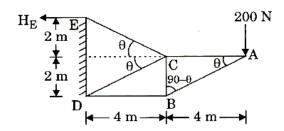
The magnitude of the horizontal support reaction at E is
