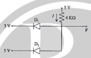
(i) For the circuit shown in the above figure using ideal diodes, find the values of the voltage V and current I indicated in the figure.
