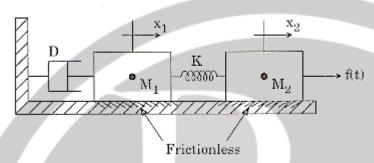
Find the state equations in matrix form for the translational mechanical system as shown above.
