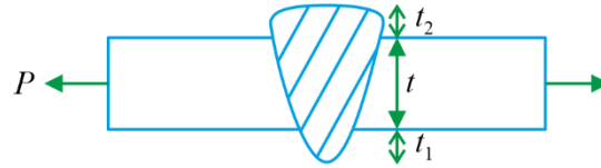
Fig.3.6: Butt weld under force P
