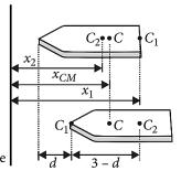
As shown in figure, let  $C_1$ ,  $C_2$  and C be the centres of mass of the boy, boat and the system (boy and boat) respectively. Let  $x_1$  and  $x_2$  be the distances of  $C_1$  and  $C_2$  from the shore. Then the centre of mass will be at a distance,
