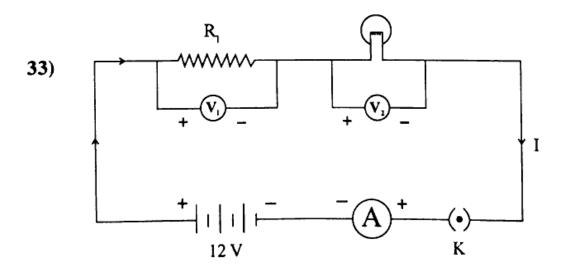
An electric lamp, whose resistance is  $25\Omega$  and a conductor of unknown resistance (R<sub>1</sub>) are connected to a 12V battery. If 0.4 A current passing through circuit. Find unknown resistance and voltage at two ends of bulb as well as the ends of unknown resistance. [3]
