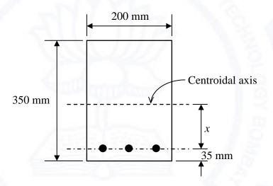
The distance of the centroidal axis from the centerline of the reinforcement (x) for the uncracked section (in mm, round off to one decimal place) is \_\_\_\_\_
