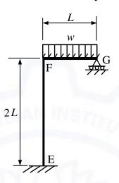
Considering the joint F being rigid, the support reaction at G is
