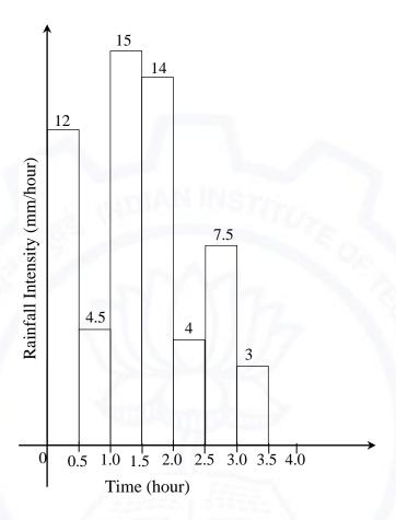
If the rainfall event has produced a direct runoff of 1.6 cm, the  $\phi$ -index of the event (in mm/hour, round off to one decimal place) would be
