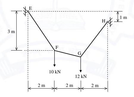
The magnitude of tension in the cable segment FG (in kN, round off to two decimal places) is \_\_\_\_\_
