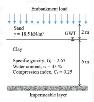
The primary consolidation settlement (in m, round off to two decimal places) of the clay layer resulting from this loading will be \_\_\_\_\_
