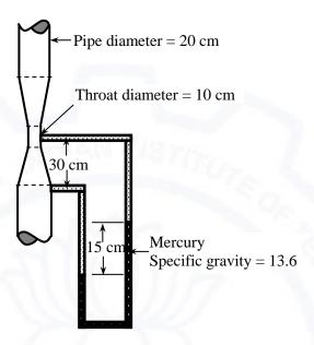
Assume  $g = 9.8 \text{ m/s}^2$ . When the deflection in the mercury manometer is 15 cm, the flow rate (in lps, round off to two decimal places) considering no loss in the venturimeter is \_\_\_\_\_
