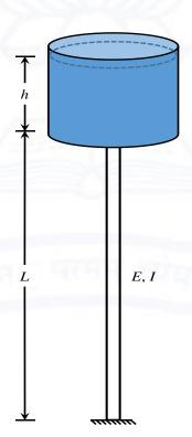
If elastic modulus (E) of steel is 200 GPa, ignoring self-weight of the tank, for the supporting steel column to remain unbuckled, the maximum depth (h) of the water permissible (in m, round off to one decimal place)
