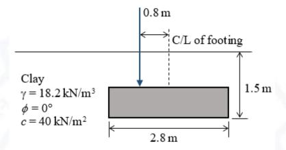
Using Meyerhoff's method, the load (in kN, round off to two decimal places) that can be applied on the footing with a factor of safety of 2.5 is
