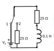
Q.51 In the circuit shown below, the output voltage Vour is \_\_\_\_\_\_ V.
