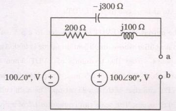
(ii) For the ladder network determine the g parameters in the s domain.
