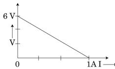
The plot of the variation of potential difference across a combination of three identical cells in series, versus current is shown below. What is the emf and internal resistance of each cell?
