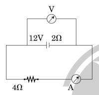
A battery of emf 12V and internal resistance 2  $\Omega$  is connected to a 4  $\Omega$  resistor as shown in the figure.
