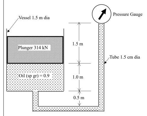
If a pressure gauge is connected with the vessel using 1.5 cm diameter tube, the reading of the gauge will be \_\_\_\_\_(in kPa, rounded off to two decimal places).
