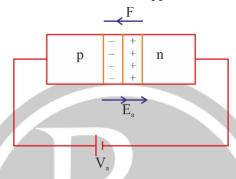
When any type of p-n junction is forward biased limiting resistance must be connected in series with the diode, the limiting resistance and diode working as potential divider network
