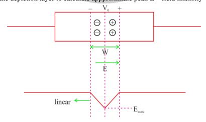
$$E_{\text{max}} = \frac{-v_0}{W/2} = \frac{-2v_0}{W} \text{ v/m}$$
