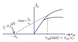
•  $r_o$  (or)  $rd = \frac{1}{slope} = \frac{v_A}{I_D} = \frac{1}{\lambda I_D}$
