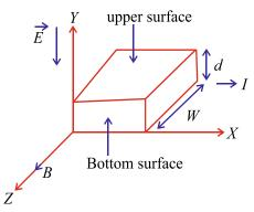
where, w = width of specimen d = height of specimen  $\text{current in } X - \text{direction} \Longrightarrow I_X$ Magnetic field in  $Z - \text{direction} = B_Z$ Field intensity in  $Y - \text{direction} = E_Y$
