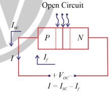
$$\begin{split} \mathbf{I} &= \mathbf{I}_{sc} - \mathbf{I}_{f} \\ V_{oc} &= \eta V_{T} \ell n \left[ \frac{\mathbf{I}_{optical}}{I_{O}} + 1 \right] \\ V_{oc} &= \eta V_{T} \ell n \left[ \frac{I_{sc}}{I_{O}} + 1 \right] \\ \\ V_{oc_{1}} - V_{oc_{2}} &= \eta V_{T} \ell n \left( \frac{I_{sc_{1}}}{I_{sc_{2}}} \right) = \eta V_{T} \ell n \left( \frac{J_{sc_{1}}}{J_{sc_{2}}} \right) \end{split}$$
