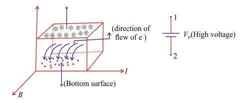
• For n-type SC bottom plate will be positively charge.
