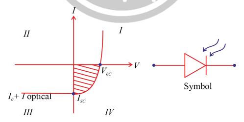
As it converts optical energy into electrical energy, it is widely use in satellite communication as a transformer. The only disadvantage of photo diode is, it has smaller power handing capacity. lubrication of PIN photo diode, which has larger power handling capacity.
