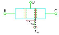
Let the depletion width for BE junction is negligible for breakdown total neutral base width =  $X_{B0}$
