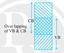
• When temperature is increased then over lapping of CB & VB also increase but there is free carrier concentration available in CB. Hence conductors have Finite amount of conductivity at 300K.
