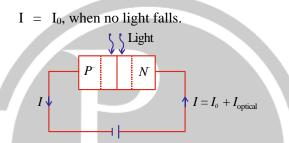
I<sub>optical</sub> → Current due to excess carriers generated due to optical energy. (Diffusion current)
