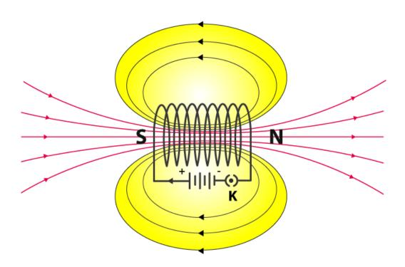
When the north pole of a bar magnet is brought close to the end of a solenoid connected to the negative terminal of a battery, the solenoid experiences a repulsive force. This repulsion occurs because like poles repel each other. From this observation, we can infer that the end of the solenoid connected to the negative terminal of the battery behaves as a north pole, while the end connected to the positive terminal acts as a south pole.
