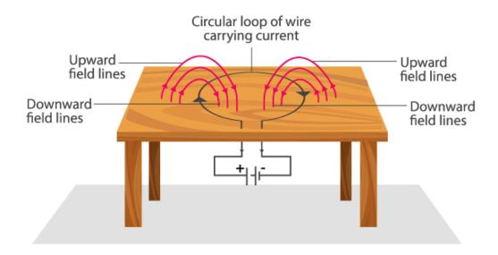
For a current flowing in a loop, the direction of the magnetic field depends on the direction of the current. If the current flows downward through the loop, the magnetic field will appear to emerge from the table surface outside the loop and merge with the table surface inside the loop.
