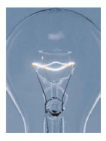
A coiled wire that becomes heated when electricity is carried through it is called a bulb's filament. This causes the filament to glow, which causes the bulb to emit light.
