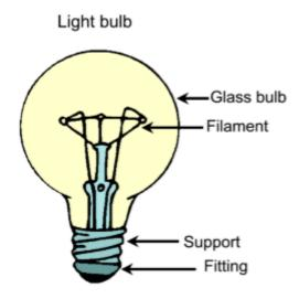
When the filament of a bulb breaks the circuit of the bulb becomes incomplete. Hence the bulb does not glow as it does not receive any electricity.
