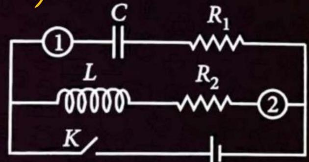
In the figure shown, a circuit contains two identical resistors with resistance  $R = 5\Omega$  and an inductance with L = 2 mH. An ideal battery of 15 V is connected in the circuit. What will be the current through the battery long after the switch is closed?
