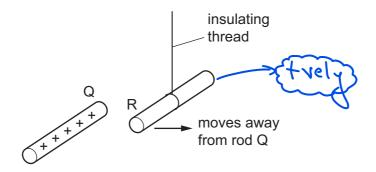
When the positively charged rod Q is brought close to rod R, rod R moves away from rod Q.
