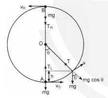
The forces acting on the body, when the string makes an angle  $\theta$  with the initial position are shown in the figure. Here, mg is the weight of body and T the tension in the string. If v be the instantaneous velocity at this point, then a centripetal force  $F = \frac{mv^2}{l}$  is required radially inward. From figure, it is clear that in equilibrium the centripetal force is provided by resultant of two forces i.e.,
