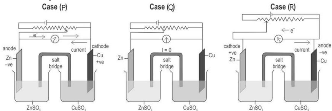
She applied external potential in all the three cells. The potential is increased slowly, till the opposing voltage reaches the value of 1.1 V.
