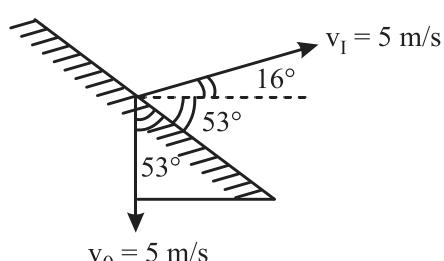
$$\begin{aligned} v_I &= (5 \cos 16^\circ) \hat{i} + (5 \sin 16^\circ) \hat{j} \\ &= (4.8 \hat{i} + 1.4 \hat{j}) \text{ m/s} \end{aligned}$$
