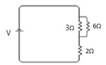
From the circuit above, it is understood that 3  $\Omega$  and 6  $\Omega$  are connected in parallel. Hence, their equivalent resistance is given by
