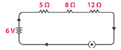
2. Redraw the circuit of Question 1, putting in an ammeter to measure the current through the resistors and a voltmeter to measure the potential difference across the 12  $\Omega$  resistor. What would be the readings in the ammeter and the voltmeter?
