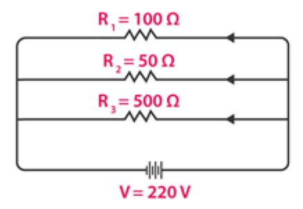
The equivalent resistance of the resistors can be calculated as follows:
