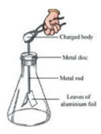
It is made up of a metal rod with a metal disc at one end and two aluminum foil leaves attached to one end. To keep the leaves safe from the ambient air, they are stored within a conical flask that has been corked.
