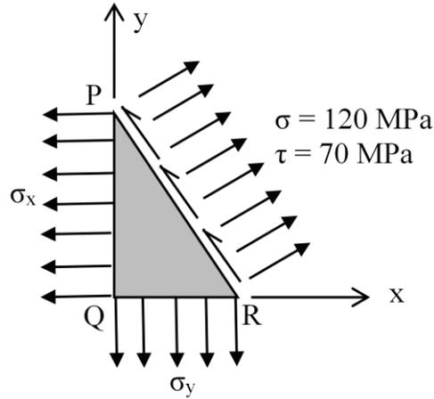
(A)  $\sigma_x = 26.7 \text{ MPa}$ ,  $\sigma_y = 172.5 \text{ MPa}$
