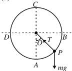
Tension at general point P, according to Newton second law of motion.
