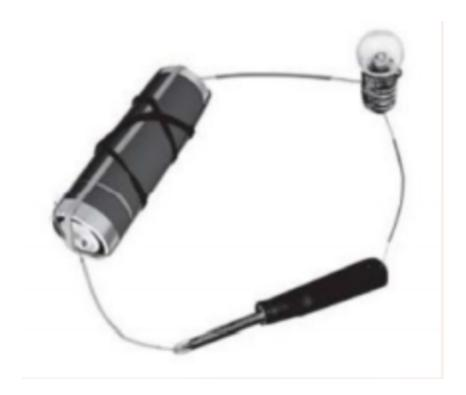
Ans: The bulb will not light since the circuit is broken due to the insulator in the middle.
