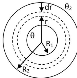
$$\frac{\Delta\theta/2}{\frac{1}{4\pi K_1} \left[ \frac{1}{R_1} - \frac{1}{R} \right]} = \frac{\Delta\theta}{\frac{1}{4\pi K_1} \left( \frac{1}{R_1} - \frac{1}{R_2} \right)}$$
