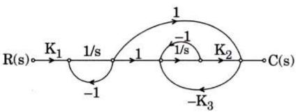
(ii) For a system represented in the figure, response to a unit step with K = 1 is given. For what value of K does the steady state error become zero?
