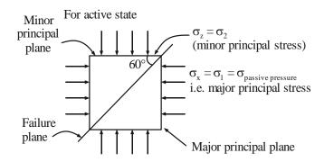
Failure plane inclination with major principal plane
