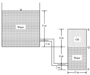
The total force (in kN) due to pressure on the side PQR of the tank is \_\_\_\_\_ (rounded off to the nearest integer').
