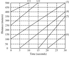
The mean speed (in km/hr) of the vehicles in the entire time-space domain is \_\_\_\_\_ (rounded off to the nearest integer).
