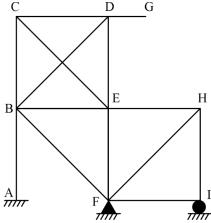
If the axial deformations are neglected, the degree of kinematic indeterminacy is (in integer').
