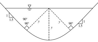
The normal depth of flow, y (in meters) for carrying a discharge of 20 m³/s is \_\_\_\_\_ (rounded off to 2 decimal places).
