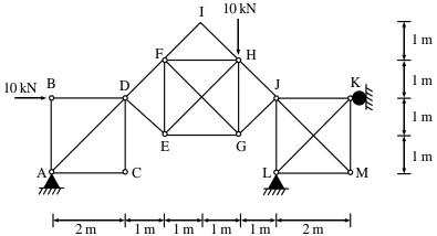
The magnitude of the reaction (in kN) at the pin support L is (rounded off to 1 decimal place).
