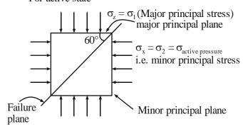
Failure plane inclination with major principal plane (horizontal)
