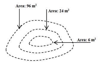
The contour interval is 1 m. Using prismoidal method, the volume of the earth needed to fill the land depression is  $m^3$ .
