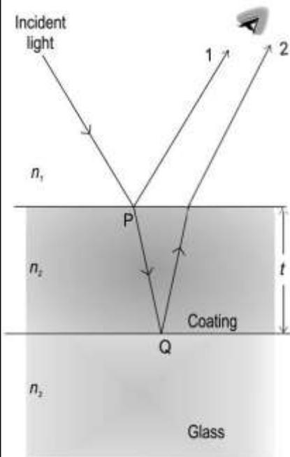
Reflected light undergoes a  $180^\circ$  phase shift when it falls on a denser medium from a rarer medium and no phase shift when it falls on a rarer medium from a denser medium. (Note: The thickness of coating is much less than the glass.)
