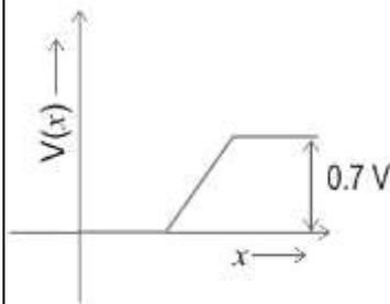
Plot a comparative graph of the potential barrier ( $V$ ) vs width of the depletion region ( $x$ ) of  $D_1$  at room temperature when the voltage at A is negative with respect to voltage at centre tap. Give reason.
