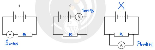
In which of the circuits does the ammeter measure the current in the resistor?
