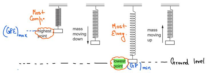
At which point is the least energy in the gravitational potential store of the mass and at which point is the most energy in the elastic store of the spring?
