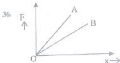
Two wires A and B of same length are made of same material. Load ( $F$ ) vs. elongation ( $x$ ) graph for these two wires is shown in the figure. Then which of the following statement(s) is/are true ?
