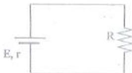
A battery of emf  $E$  and internal resistance  $r$  is connected with an external resistance  $R$  as shown in the figure. The battery will act as a constant voltage source if
