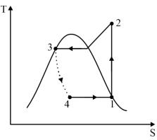
From figure it is seen that process 1-2 is isentropic compression and the curved is vertically straight in nature.
