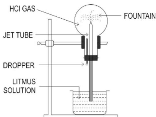
The fountain starts when a few drops of water from the dropper are introduced into the flask. Instead of the drops of water, Pooja started the fountain by introducing a few drops of Sodium hydroxide into the flask.
