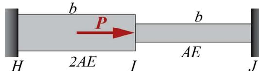
To make the axial force in rod  $HI$  equal to zero, the value of the external force  $P$  (in **N**) is \_\_\_\_\_. (round off to the nearest integer)
