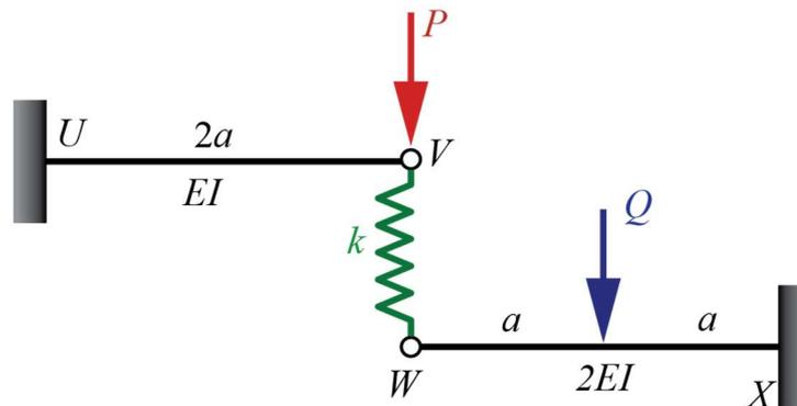
The magnitude of force  $Q$  (in **kN**) is \_\_\_\_\_. (round off to the nearest integer)
