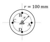
The rotor is driven by a motor at uniform angular speed of 10 rad/s. If one of the masses gets detached then the magnitude of the resultant unbalance force on the rotor is \_\_\_\_\_\_N (round off to 2 decimal places).
