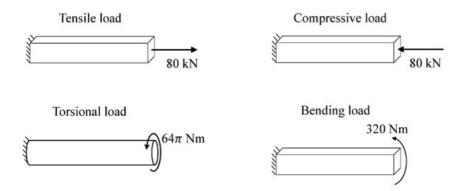
Which specimen(s) will fail due to the applied load as per maximum shear stress theory?
