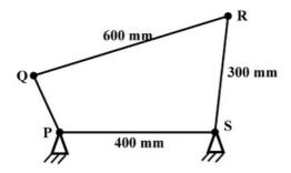
For the mechanism to be a crank-rocker mechanism, the length of the link PQ can be
