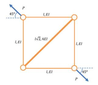
The smallest value of P, at which any of the truss members will buckle is
