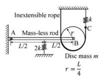
Neglecting the influence of gravity, the natural frequency of the system for small amplitude vibration is
