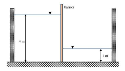
Taking the density of water as  $1000 \text{ kg/m}^3$ , and the acceleration due to gravity as  $10 \text{ m/s}^2$ , the maximum absolute bending moment developed in the cantilever is \_\_\_\_\_\_ kN·m (round off to the nearest integer).
