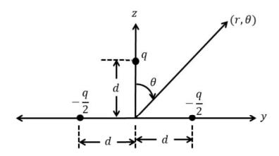
For r = 10 m;  $\theta = 60$  degrees;  $q = 10^{-6}$  Coulomb, and  $d = 10^{-3}$  m, the electric dipole potential in volts (rounded off to three decimal places) at a point  $(r, \theta)$  is
