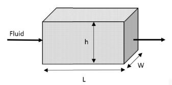
An incompressible fluid having a viscosity of 2 cP is flowing through a porous medium at the inlet and exit pressures of  $7 \times 10^6$  Pa and  $6 \times 10^6$  Pa, respectively.
