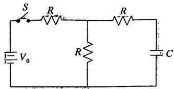
The capacitor is initially uncharged. At time t = 0, the switch S is closed. The voltage across the capacitor as a function of time t for t > 0 is given by
