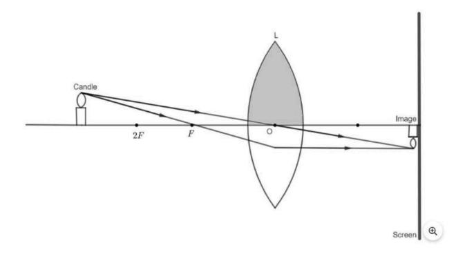
Let us consider a convex lens that has a black paper coating on half of it. We maintain a screen on one side of the lens and a burning candle on the other.
